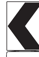
18" x 24" Sign (Maximum Sign Dimension) Chevron CWI-8, Opposing Traffic Lane Divider, Driveway sign D70a, Keep Right R4 series or other signs as approved by Engineer
