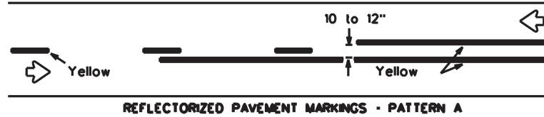
REFLECTORIZED PAVEMENT MARKINGS - PATTERN A
