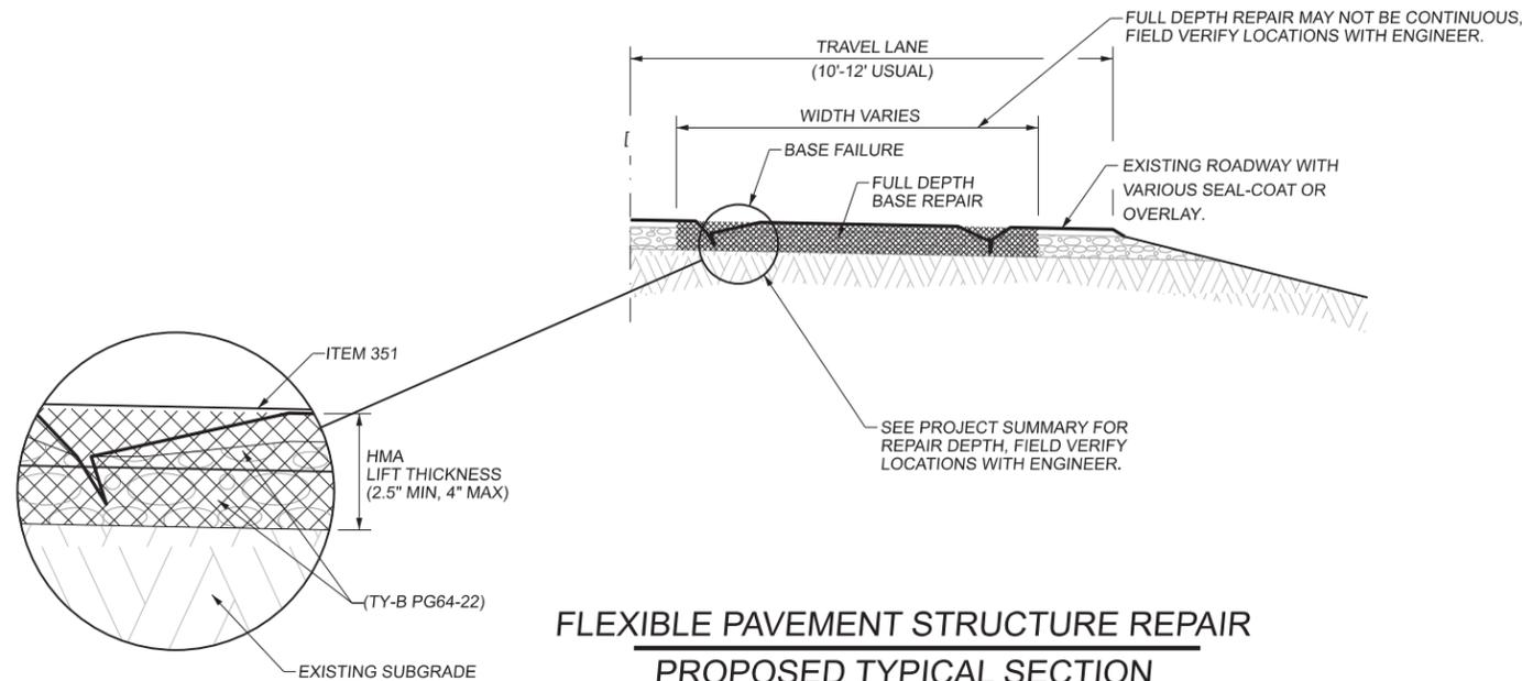
**FLEXIBLE PAVEMENT STRUCTURE REPAIR
