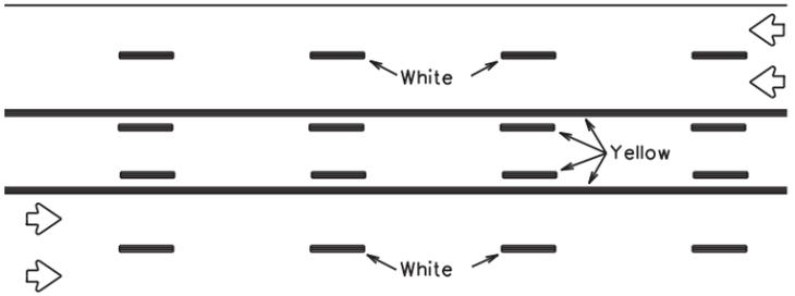
REFLECTORIZED PAVEMENT MARKINGS
