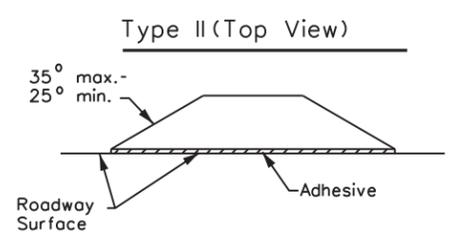
**SECTION A REFLECTORIZED RAISED PAVEMENT MARKER (RPM)**
