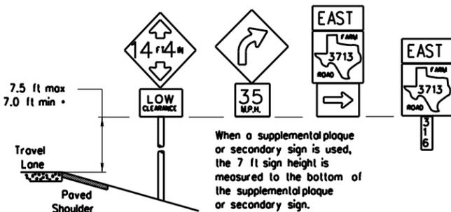
When a supplemental plaque or secondary sign is used, the 7 ft sign height is measured to the bottom of the supplemental plaque or secondary sign.
