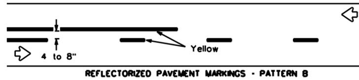
Pattern A is the TxDOT Standard, however Pattern B may be used if approved by the Engineer. Prefabricated markings may be substituted for reflectORIZED pavement markings.
