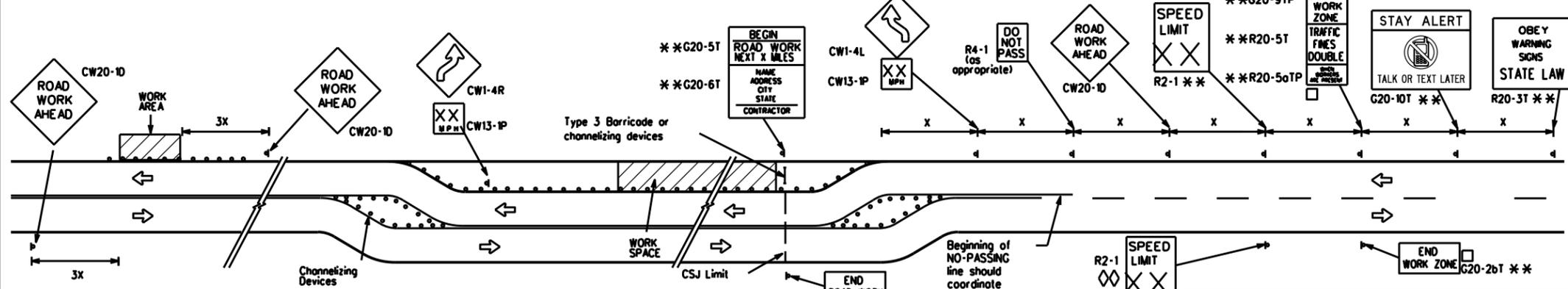
When extended distances occur between minimal work spaces, the Engineer/Inspector should ensure additional "ROAD WORK AHEAD" (CW20-1D) signs are placed in advance of these work areas to remind drivers they are still within the project limits. See the applicable TCP sheets for exact location and spacing of signs and channelizing devices.
