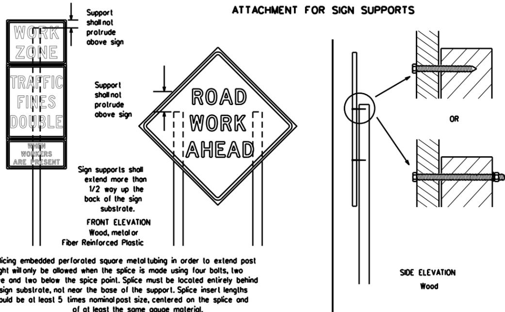
Nois shall NOT be allowed. Each sign shall be attached directly to the sign support. Multiple signs shall not be joined or spliced by any means. Wood supports shall not be extended or repaired by splicing or other means.
