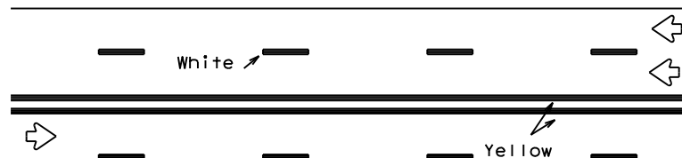
REFLECTORIZED PAVEMENT MARKINGS
