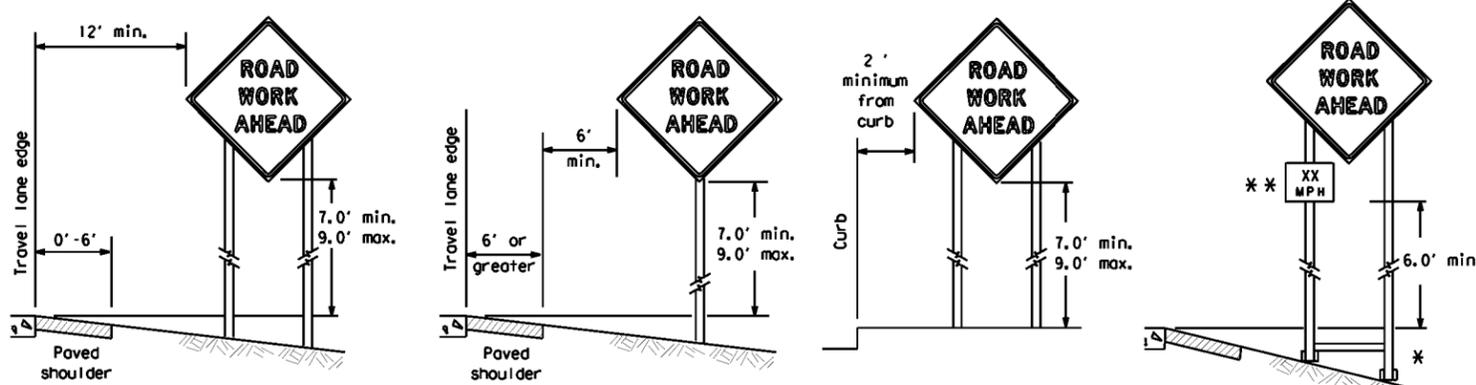
\* When placing skid supports on unlevel ground, the leg post lengths must be adjusted so the sign appears straight and plumb. Objects shall NOT be placed under skids as a means of leveling.
