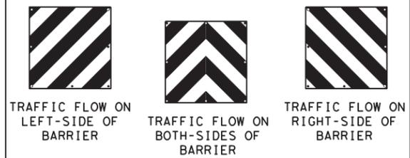
\* NOTE: ENGINEER OR CONTRACTOR SHALL COORDINATE WITH THE MANUFACTURER FOR THE CORRECT DECAL PER TRAFFIC FLOW, LEFT, RIGHT OR BOTH-SIDES.
