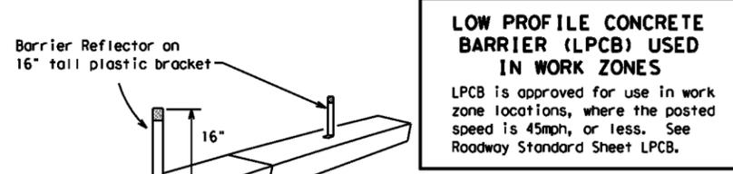
Max. spacing of barrier reflectors is 20 feet. Attach the delineators as per manufacturer's recommendations.
