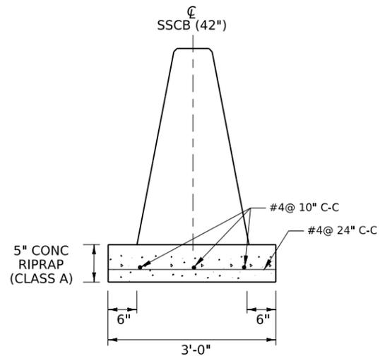
**SSCB & CONCRETE RIPRAP DETAIL**
