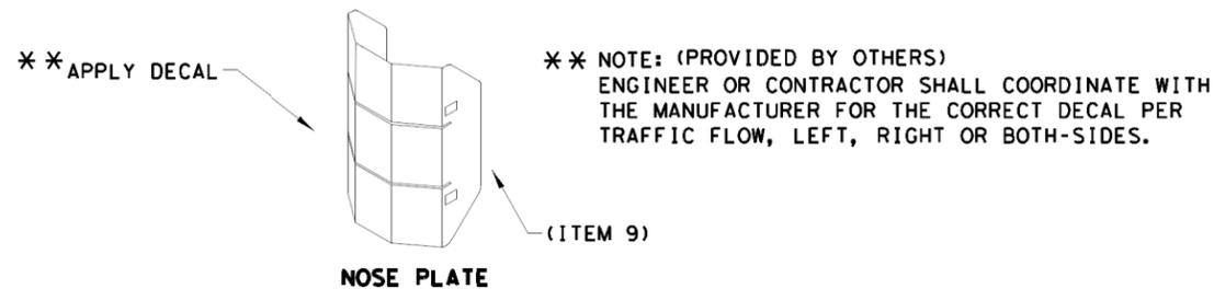
NOTE: APPLY A HIGH REFLECTIVE DECAL TO THE NOSE PLATE. DELINEATION DECAL ORIENTATION IS SHOWN ON THE CONSTRUCTION PLAN SET AND SHALL BE IN ACCORDANCE WITH THE TEXAS MUTCD FOR (TRAFFIC CONTROL DEVICES). DECALS ARE AVAILABLE FOR TRAFFIC FLOW ON THE LEFT-SIDE, BOTH -SIDES AND RIGHT-SIDE.
