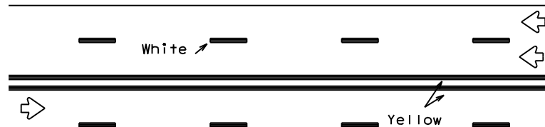
REFLECTORIZED PAVEMENT MARKINGS
