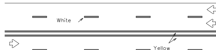
REFLECTORIZED PAVEMENT MARKINGS
