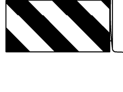
12" x 24" Vertical Panel mount with diagonals sloping down towards travel way
