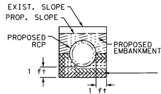
**REINFORCED CONCRETE PIPE (NON-ROADBED) BACKFILL DETAIL**
