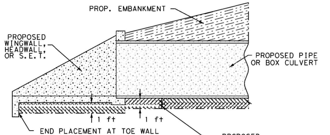
**CAST IN PLACE END TREATMENT BACKFILL DETAIL**
