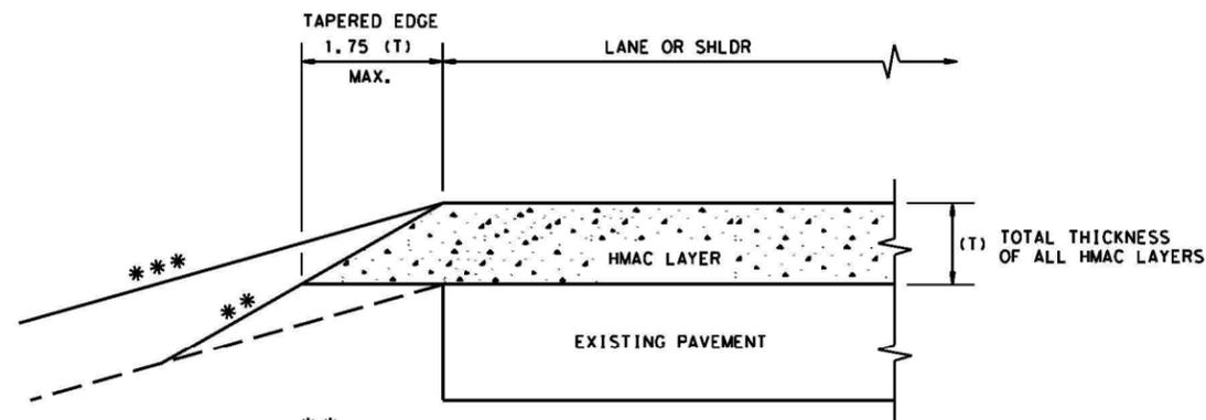
\*\* EXISTING ROADSIDE EMBANKMENT TO BE GRADED TO PRODUCE A SMOOTH LEVEL SURFACE FOR PLACEMENT OF TAPERED EDGE. THIS WORK IS SUBSIDIARY TO THE VARIOUS BID ITEMS.
