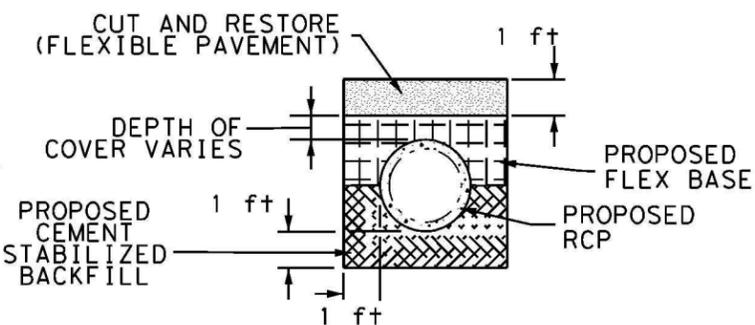
**REINFORCED CONCRETE PIPE BACKFILL CUT AND RESTORE PAVEMENT DETAIL**
