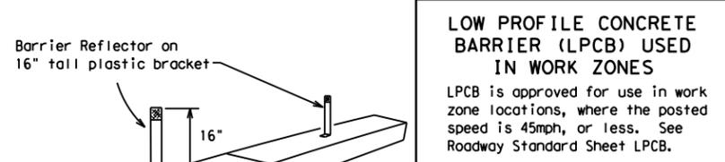
**LOW PROFILE CONCRETE BARRIER (LPCB) USED IN WORK ZONES**
