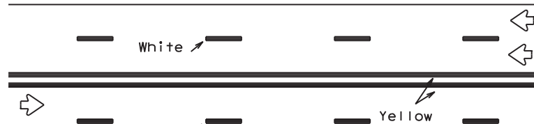
REFLECTORIZED PAVEMENT MARKINGS
