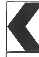
18" x 24" Sign (Maximum Sign Dimension) Chevron CW1-B, Opposing Traffic Lane Divider, Driveway sign D70a, Keep Right R4 series or other signs as approved by Engineer
