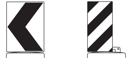
18" x 24" Sign (Maximum Sign Dimension) Chevron CW1-8, Opposing Traffic Lane Divider, Driveway sign D70a, Keep Right R4 series or other signs as approved by Engineer 12" x 24" Vertical Panel mount with diagonals sloping down towards travel way
