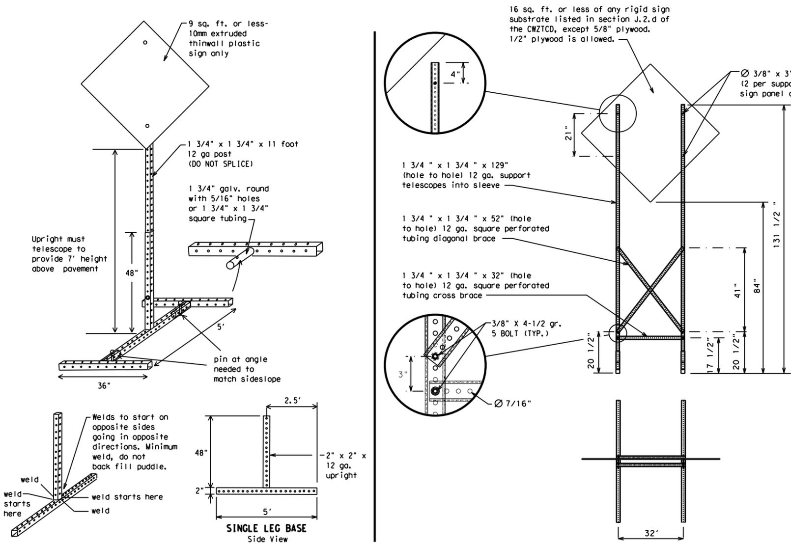
**SKID MOUNTED PERFORATED SQUARE STEEL TUBING SIGN SUPPORTS**
