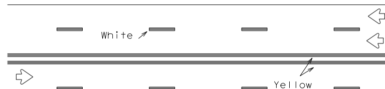
REFLECTORIZED PAVEMENT MARKINGS
