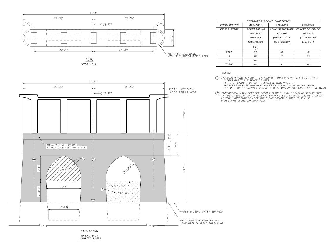
NOTE: SHADING DENOTES LIMITS FOR PENETRATING CONCRETE SURFACE TREATMENT
