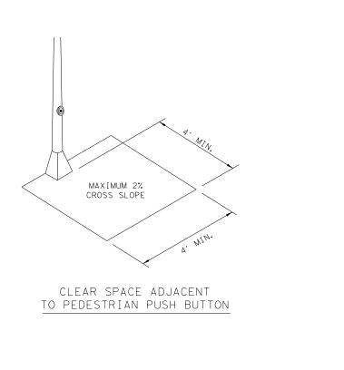
OF MORE THAN 4" INTO THE PEDESTRIAN CIRCULATION AREA, CONSTRUCT ADDITIONAL CURB OR FOUNDATION AT THE BOTTOM TO PROVIDE A MAXIMUM 4" OVERHANG.
