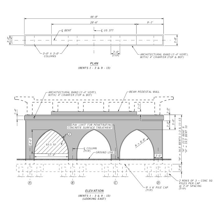
NOTE: SHADING DENOTES LIMITS FOR PENETRATING CONCRETE SURFACE TREATMENT
