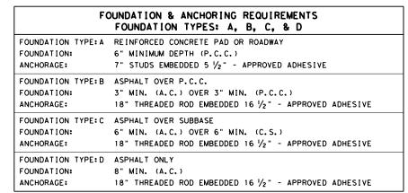
ASPHALT CONCRETE (A.C.) COMPACTED SUBBASE (C.S.) PORTLAND CEMENT CONCRETE (P.C.C.)
