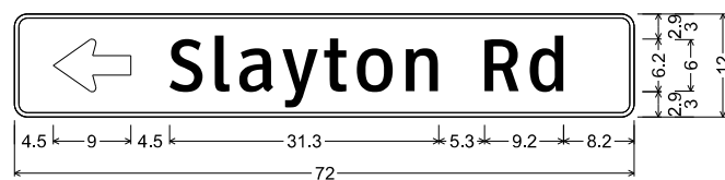
D21-1TL_VARx12; 1.5" Radius, 0.5" Border, White on Green; Standard Arrow Custom 9.0" X 6.1" 180°; "Slayton Rd", ClearviewHwy-3-W;
