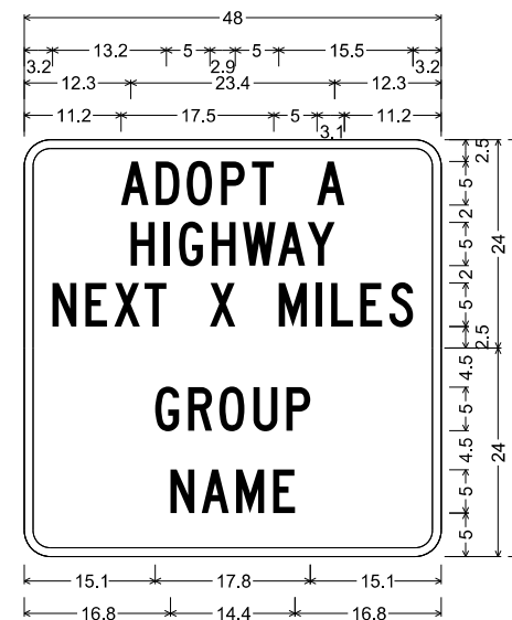
D14-4T-2_48x48; 3.0" Radius, 1.0" Border, White on Blue; "ADOPT A", C; "HIGHWAY", C; "NEXT X MILES", C; 3.0" Radius, 1.0" Border, White on Blue; "GROUP", C; "NAME", C;
