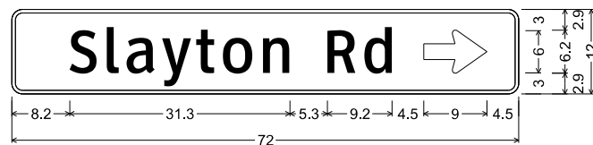
D21-1TR_VARx12; 1.5" Radius, 0.5" Border, White on Green; "Slayton Rd", ClearviewHwy-3-W; Standard Arrow Custom 9.0" X 6.1" 0°;
