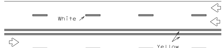
REFLECTORIZED PAVEMENT MARKINGS
