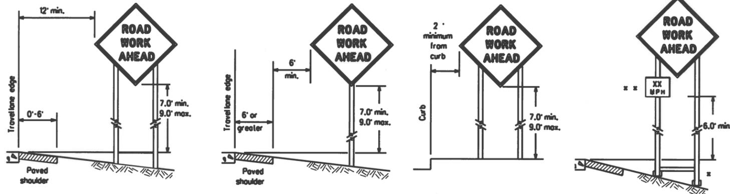
\* When placing skid supports on uneven ground, the leg post lengths must be adjusted so the sign appears straight and plumb. Objects shall NOT be placed under skids as a means of leveling.
