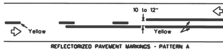
REFLECTORIZED PAVEMENT MARKINGS - PATTERN A
