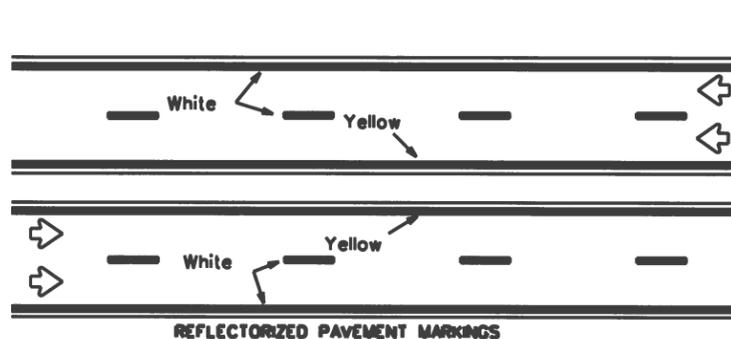
REFLECTORIZED PAVEMENT MARKINGS
