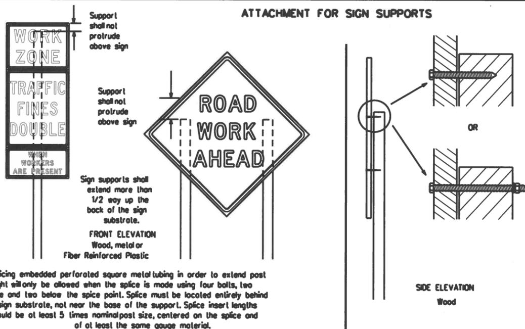
Attachment to wooden supports will be by bolts and nuts or screws. Use TxDOT's or manufacturer's recommended procedures for attaching sign substrates to other types of sign supports
