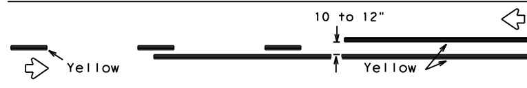
REFLECTORIZED PAVEMENT MARKINGS - PATTERN A
