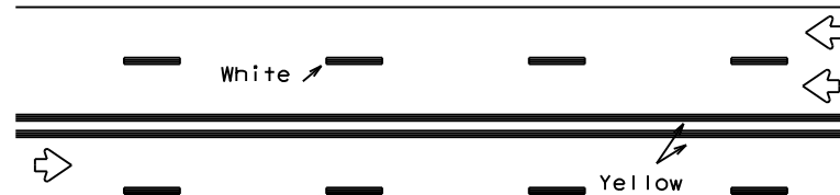
REFLECTORIZED PAVEMENT MARKINGS
