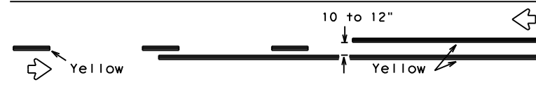
REFLECTORIZED PAVEMENT MARKINGS - PATTERN A
