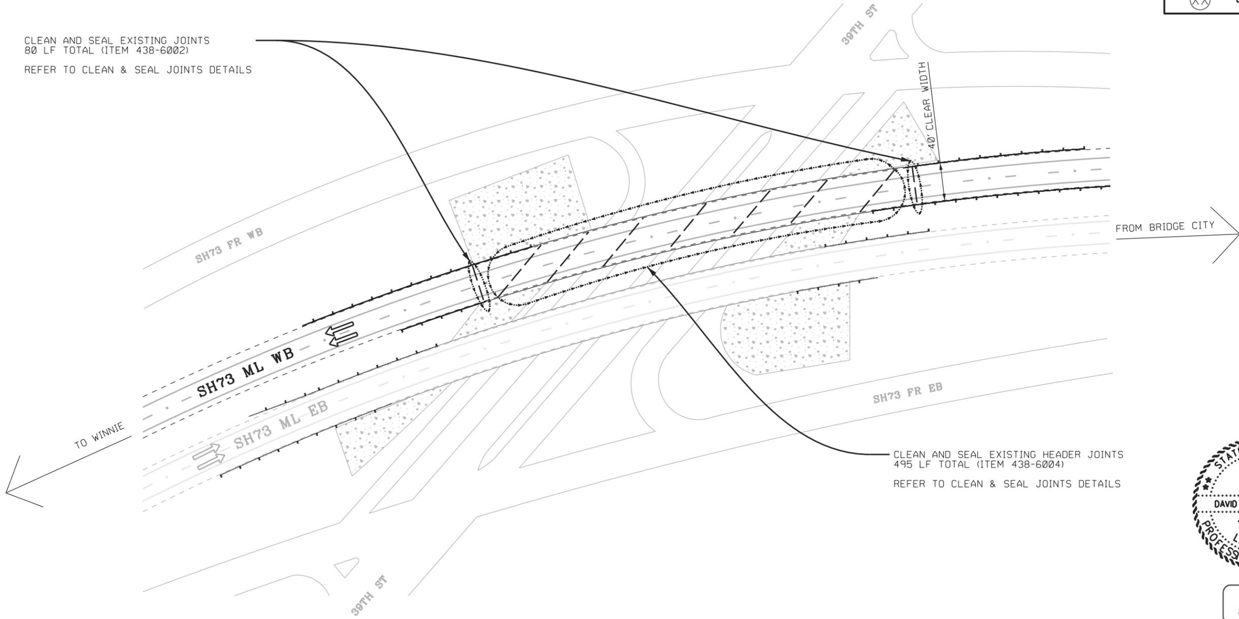
CLEAN AND SEAL EXISTING HEADER JOINTS
