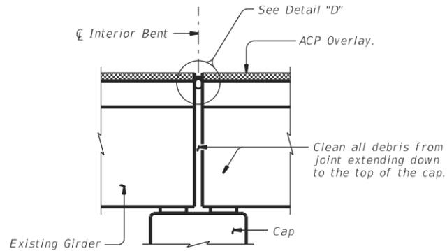
**HEADER JOINT WITH SILICONE SEAL**
