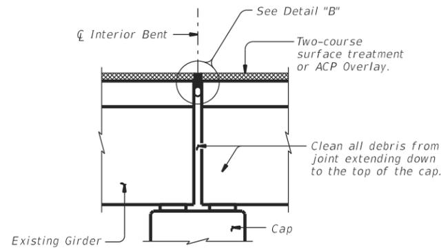
**JOINT WITH HOT Poured RUBBER SEAL**
