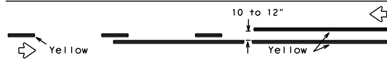
REFLECTORIZED PAVEMENT MARKINGS - PATTERN A
