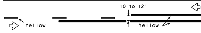
REFLECTORIZED PAVEMENT MARKINGS - PATTERN A
