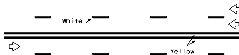
REFLECTORIZED PAVEMENT MARKINGS
