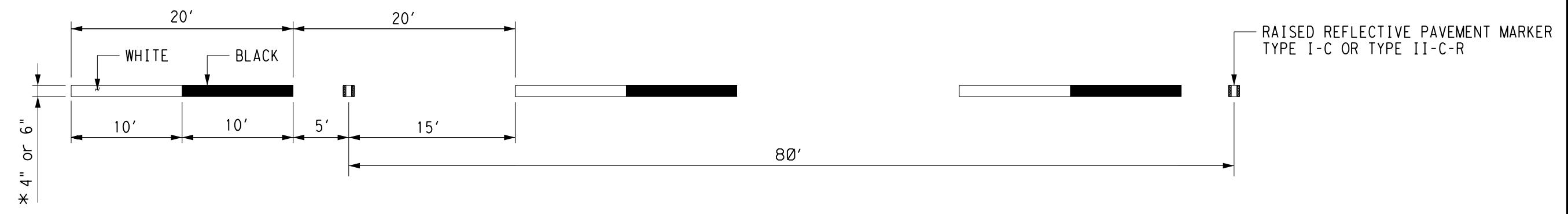
CONTRAST LANE LINES USING LIQUID APPLICATIONS (MULTIPOLYMER, THERMOPLASTIC, ETC.)
