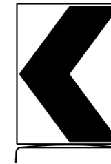
18" x 24" Sign (Maximum Sign Dimension) Chevron CWI-8, Opposing Traffic Lane Divider, Driveway sign D70a, Keep Right R4 series or other signs as approved by Engineer
