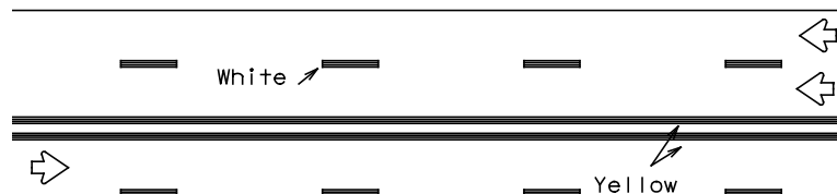
REFLECTORIZED PAVEMENT MARKINGS
