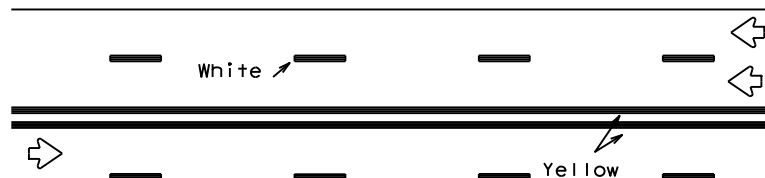
REFLECTORIZED PAVEMENT MARKINGS
