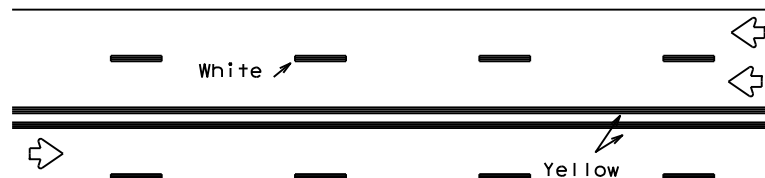
REFLECTORIZED PAVEMENT MARKINGS
