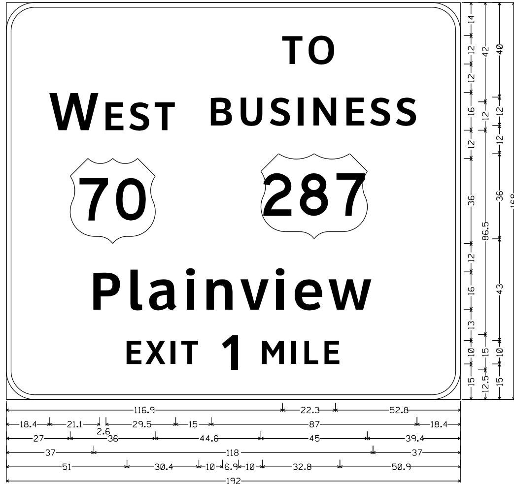
12.0' Radius, 2.0' Border, White on Green; 'TO', ClearviewHwy-5-W-R; 'W EST', ClearviewHwy-5-W-R; US 70 M1-4; 'BUSINESS', ClearviewHwy-5-W-R; US 287 M1-4; 'Plainview', ClearviewHwy-5-W-R; 'EXIT', ClearviewHwy-5-W-R; '1', ClearviewHwy-5-W-R; 'MILE', ClearviewHwy-5-W-R;
