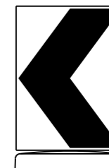
18" x 24" Sign (Maximum Sign Dimension) Chevron CW1-8, Opposing Traffic Lane Divider, Driveway sign D70a, Keep Right R4 series or other signs as approved by Engineer
