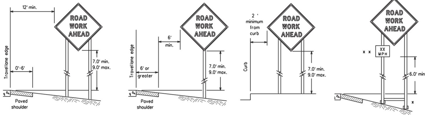
x When placing skid supports on unlevel ground, the leg post lengths must be adjusted so the sign appears straight and plumb. Objects shall NOT be placed under skids as a means of leveling.
