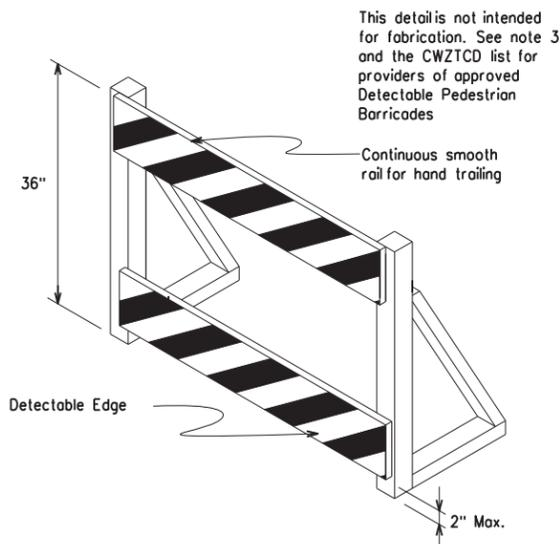
This detail is not intended for fabrication. See note 3 and the CWZTCD list for providers of approved Detectable Pedestrian Barricades
