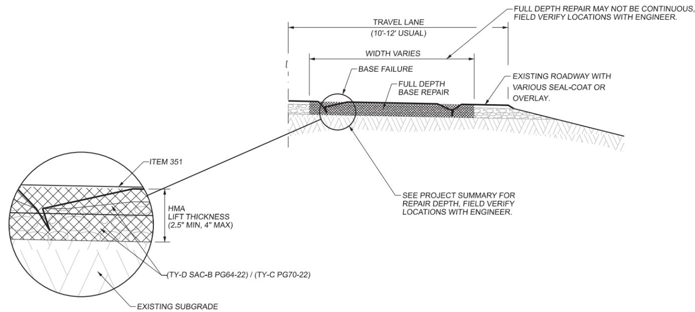
**FLEXIBLE PAVEMENT STRUCTURE REPAIR
