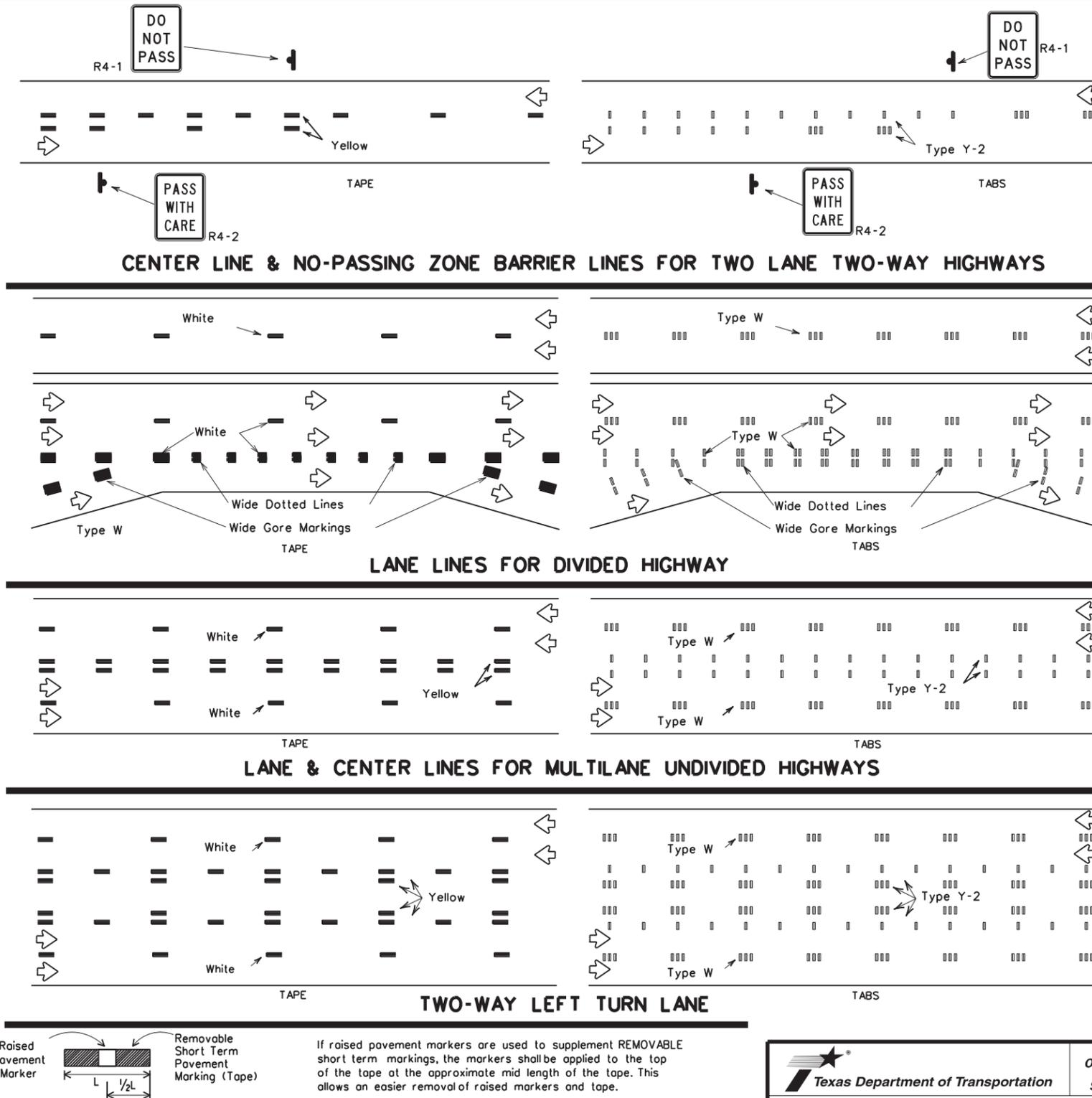
**PREFABRICATED PAVEMENT MARKINGS**
