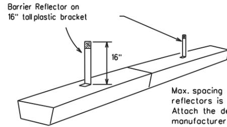
**LOW PROFILE CONCRETE BARRIER (LPCB) USED IN WORK ZONES**
