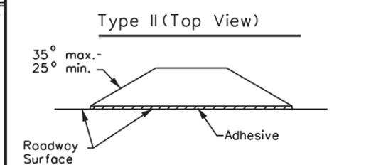
**SECTION A REFLECTORIZED RAISED PAVEMENT MARKER (RPM)**
