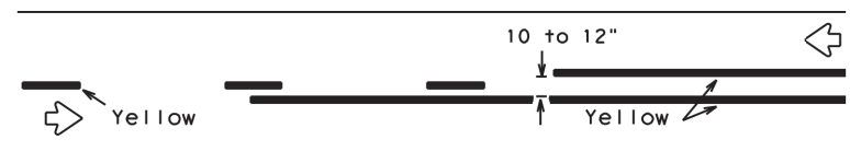
REFLECTORIZED PAVEMENT MARKINGS - PATTERN A
