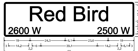
D3-1G(7) 12ft; 1.5" Radius, 1.0" Border, White on Green; "Red Bird", ClearviewHwy-3-W; "2600 W", ClearviewHwy-3-W; "2500 W", ClearviewHwy-3-W;
