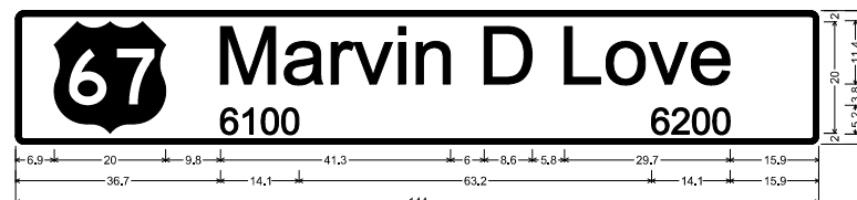
D3-1G(7) 12ft; 1.5" Radius, 1.0" Border, White on Green; "Marvin D Love", ClearviewHwy-3-W; "6100", ClearviewHwy-3-W; "6200", ClearviewHwy-3-W;
