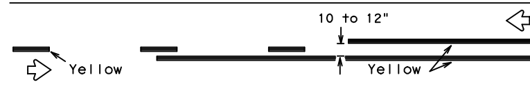
REFLECTORIZED PAVEMENT MARKINGS - PATTERN A
