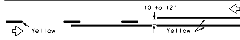
REFLECTORIZED PAVEMENT MARKINGS - PATTERN A
