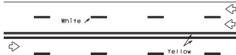
REFLECTORIZED PAVEMENT MARKINGS
