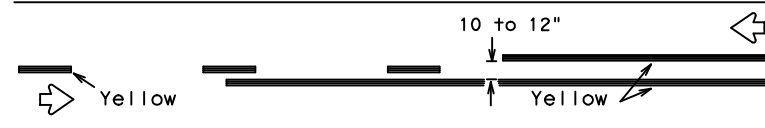
REFLECTORIZED PAVEMENT MARKINGS - PATTERN A
