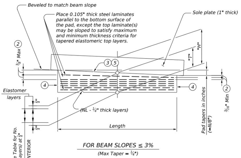
**LAMINATED ELASTOMERIC BEARING PAD DETAILS**
