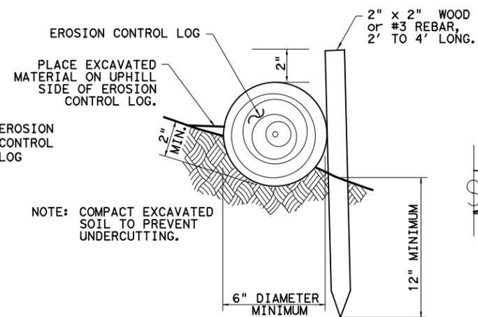
**STAKE AND LASHING ANCHORING DETAIL**
