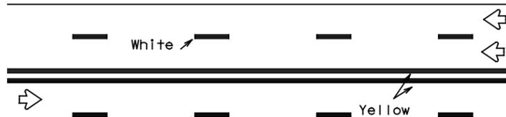
REFLECTORIZED PAVEMENT MARKINGS
