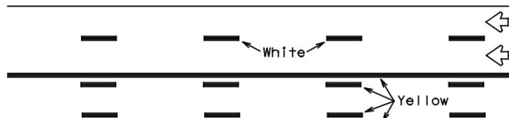
REFLECTORIZED PAVEMENT MARKINGS
