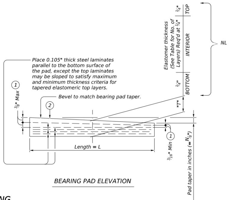
BEARING PAD ELEVATION
