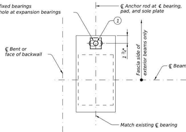
**BEARING PLACEMENT AND ANCHOR ROD DETAILS**
