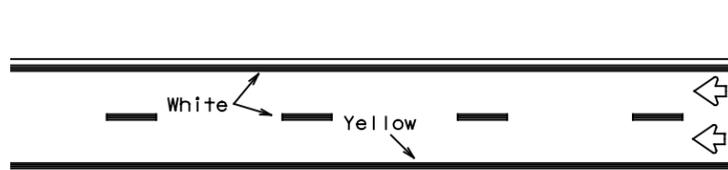
REFLECTORIZED PAVEMENT MARKINGS
