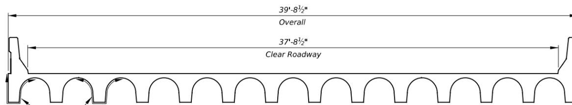
② Waterproof beams to the limits shown for the length and location of repair given in the Table of Pan Girder / Stem Repairs
