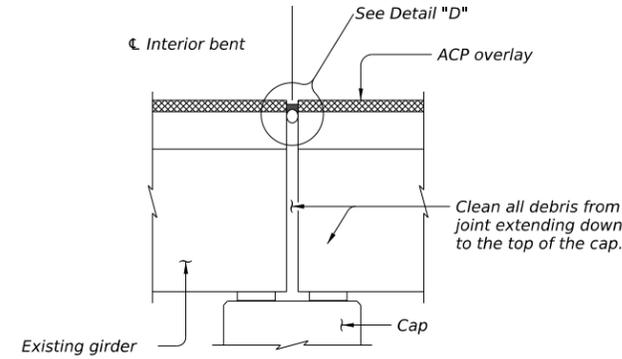
**HEADER JOINT WITH SILICONE SEAL**
