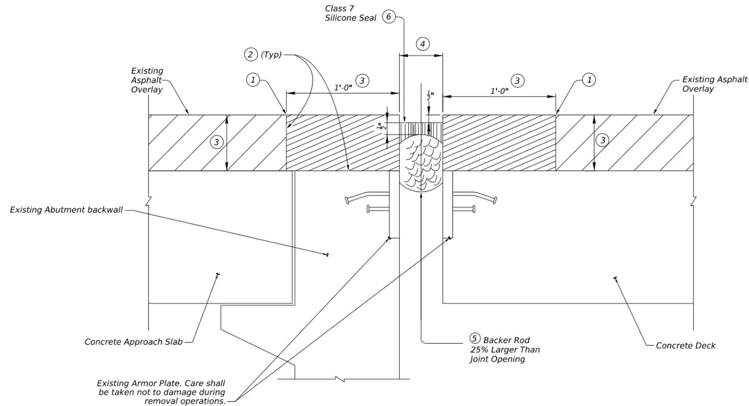
**HEADER TYPE EXPANSION JOINT REPLACEMENT DETAIL**
