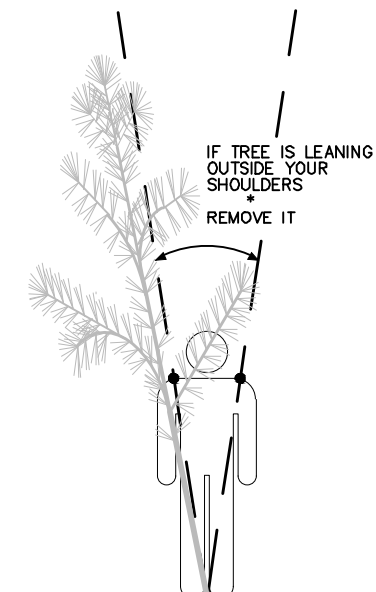
LEANING TREE REMOVAL
