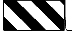
12" x 24" Vertical Panel mount with diagonals sloping down towards travel way
