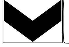
18" x 24" Sign (Maximum Sign Dimension) Chevron CWI-8, Opposing Traffic Lane Divider, Driveway sign 070a, Keep Right R4 Series or other signs as approved by Engineer
