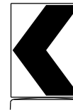
18" x 24" Sign (Maximum Sign Dimension) Chevron CW-8, Opposing Traffic Lane Divider, Driveway sign D70a, Keep Right R4 series or other signs as approved by Engineer
