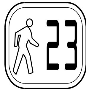
PEDESTRIAN HEAD (ONE-SECTION HEAD DISPLAYS WALK AND DON'T WALK SYMBOLS AND COUNTDOWN MODULE)
