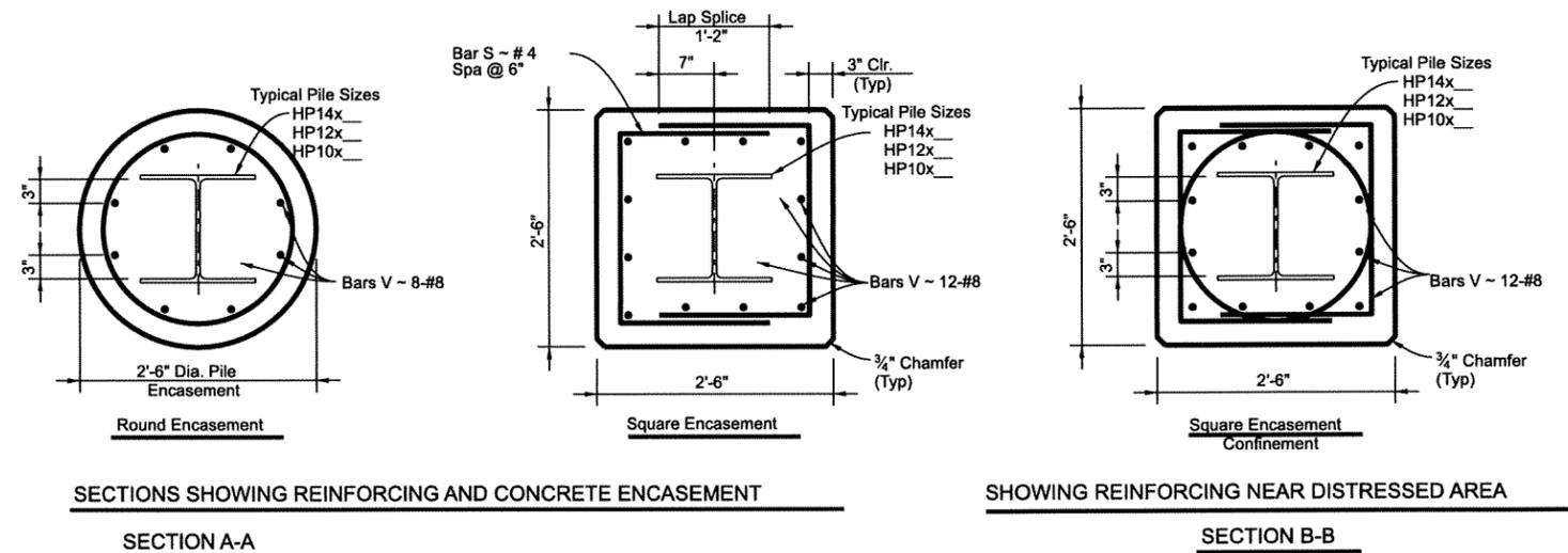
SECTIONS SHOWING REINFORCING AND CONCRETE ENCASEMENT
