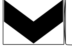
18" x 24" Sign (Maximum Sign Dimension) Chevron CWI-8, Opposing Traffic Lane Divider, Driveway sign D70a, Keep Right R4 Series or other signs as approved by Engineer
