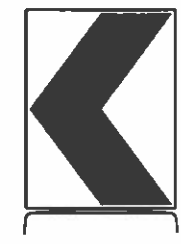
18" x 24" Sign (Maximum Sign Dimension) Chevron CWI-8, Opposing Traffic Lane Divider, Driveway sign D70a, Keep Right R4 series or other signs as approved by Engineer
