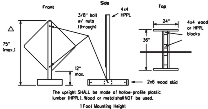
Attachment to wooden supports will be by bolts and nuts or screws. Use TxDOT's or manufacturer's recommended procedures for attaching sign substrates to other types of sign supports.
