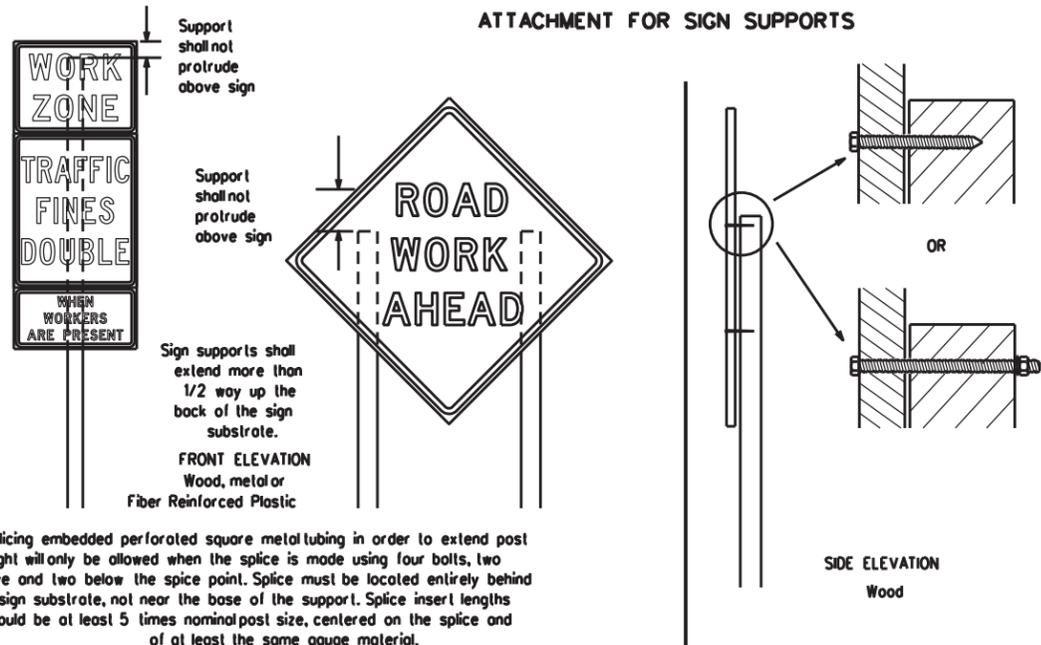
Splicing embedded perforated square metal tubing in order to extend post height will only be allowed when the splice is made using four bolts, two above and two below the splice point. Splice must be located entirely behind the sign substrate, not near the base of the support. Splice insert lengths should be at least 5 times nominal post size, centered on the splice and of at least the same gauge material.
