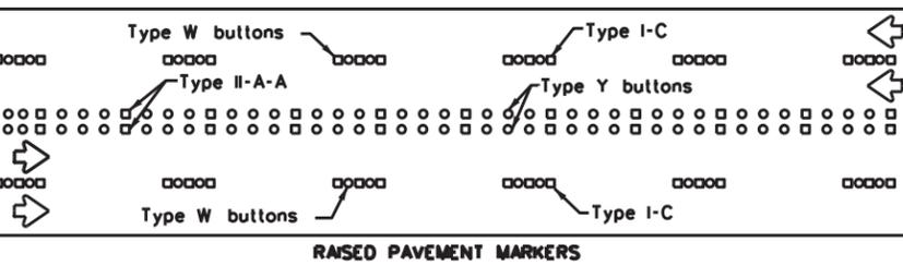
Prefabricated markings may be substituted for reflectORIZED pavement markings.
