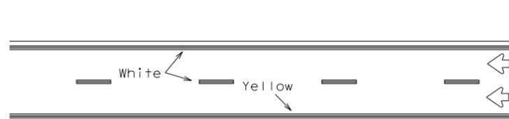
REFLECTORIZED PAVEMENT MARKINGS
