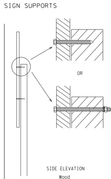
Attachment to wooden supports will be by bolts and nuts or screws. Use TxDOT's or manufacturer's recommended procedures for attaching sign substrates to other types of sign supports
